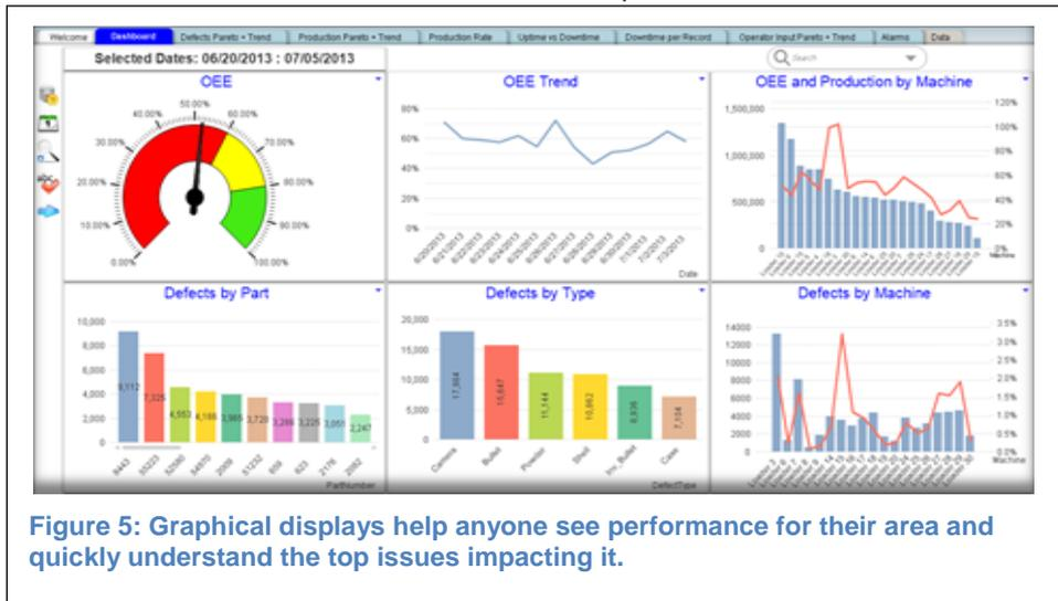
equipment effectiveness (OEE) in the top three panes, and quality defects in the bottom three. At a glance, you can see current performance, trends, and where problems most commonly occur. Additionally, employees can click on a chart and drill down to see more detail, or switch to a different slice of data.
